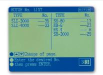
Key rotor specifications are stored in memory and can be conveniently recalled and viewed on the LCD screen.
