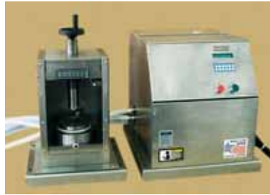
Special "all stainless steel" AutoPellet Press for corrosive operating environment.
