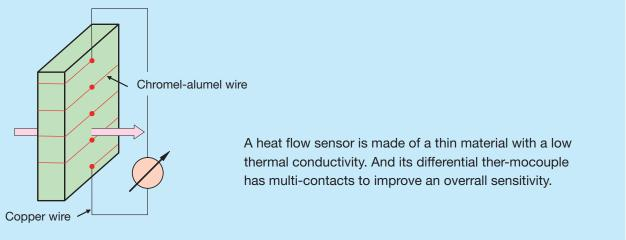
Construction of Heat Flow Sensor
