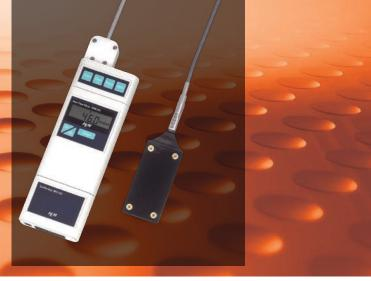
Easy to carry, a portable type Heat Flow Meter. To check heat dissipation from boilers or steam piping, evaluate thermal insulation, measure heating value of electronic devices and components, detect flaws of blast furnaces, etc. This Heat Flow Meter can be used at various sites on various occasions.
