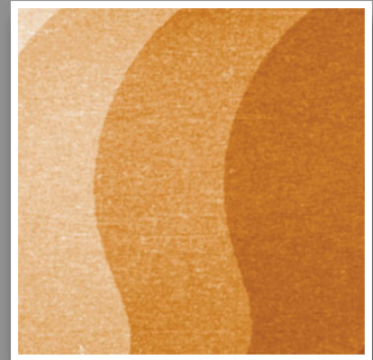
Silicon Test Echelon Pattern STEPP. Monatomic step image with closed-loop on. Step height 0.31 nm. Scan size: 7x7 \mu\text{m} .
