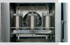
The Cryst-EX equipment is built in an Agilent GC oven where three stirred stainless steel vessels are installed. Samples are introduced manually in the crystallization vessels through a small cap before the automated analysis is initiated.
