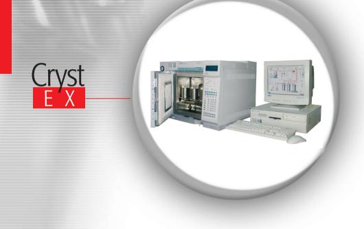
Cryst-EX is a fully automated technique for the fast and precise analysis of the Xylene Extractables / Heptane Solubles in Polypropylene resins with a simple and robust instrument. The overall analysis time is less than 3 hours. The incor-poration of an additional Infrared sensor and a single capillary viscometer makes of Cryst-EX a very powerful apparatus still being adapted to be used in a Quality Control Laboratory.
