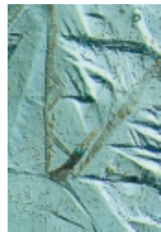
Hardened spring steel, interference contrast
