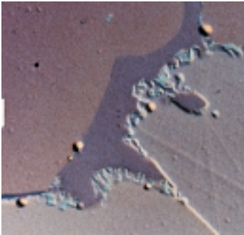
High alloy steel with interference colour layer
