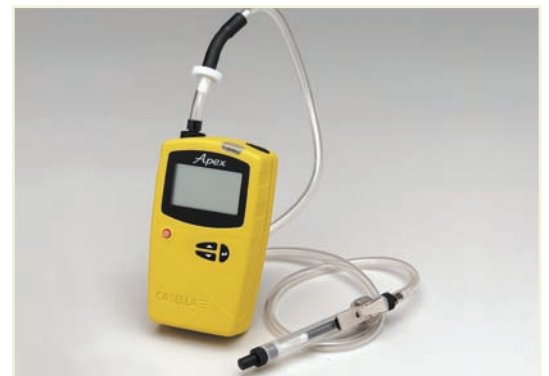
Pump with low - flow adaptor for vapour sampling
