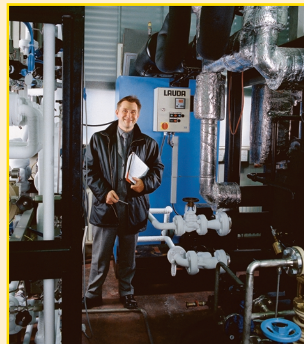
Kryopac system on the test bench. If theory and practise are in harmony, it is a pleasure for the inventor. Operating temperature from -100 up to 200 °C Cooling capacity 18 kW/-100 °C Type KP 350 HK
