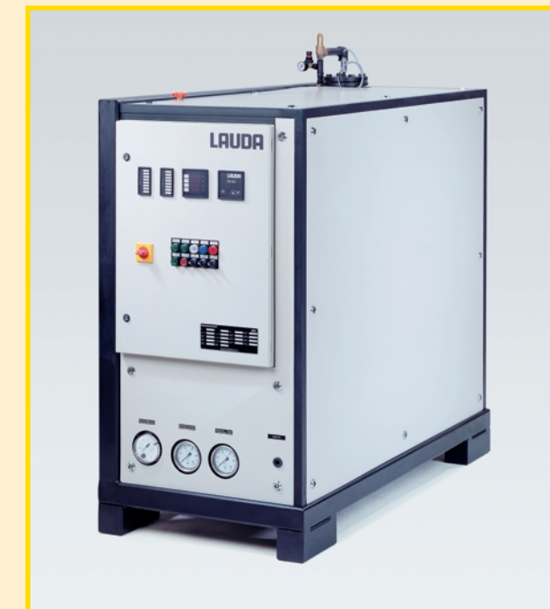
Process cooling unit with water-cooled condenser to control the temperature within a temperature range from -70 up to 150 °C. Cooling capacity 2 kW/-70 °C Additional electric heating 12 kW Type SUK 350 W II
