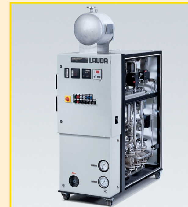
Flexible heat transfer unit in stainless steel for the temperature control of different consumer circuits in a temperature range from -30 up to 160 °C. Heating capacity 50 kW Type ITHW 350
