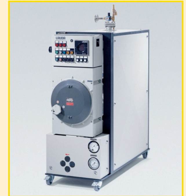
Heat transfer unit with water-cooled heat exchanger for the temperature control of a reactor in a temperature range from 20 up to 350 °C for installation in hazardous areas. Heating capacity 48 kW Type ITH 350 Ex
