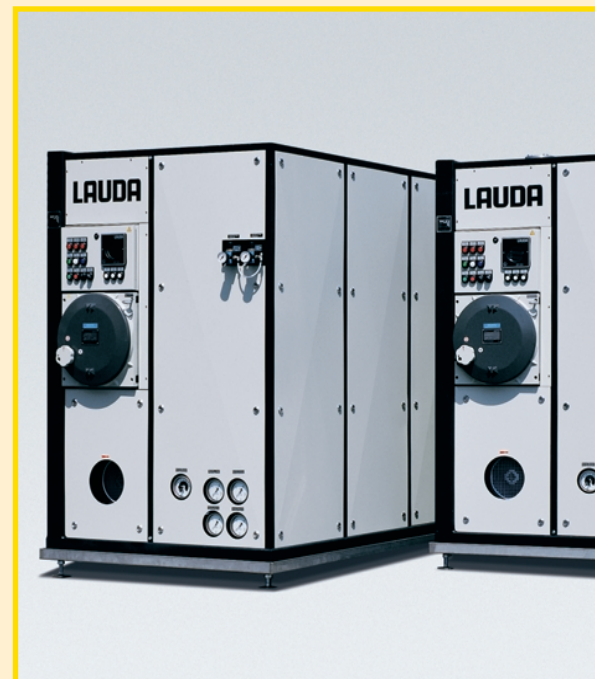
Process cooling unit with water-cooled condenser for installation in hazardous area to control the temperature within a temperature range from -30 up to 150 °C. Cooling capacity 300 kW/0 °C Additional heating steam 500 kW Type SUK 600 W Ex
