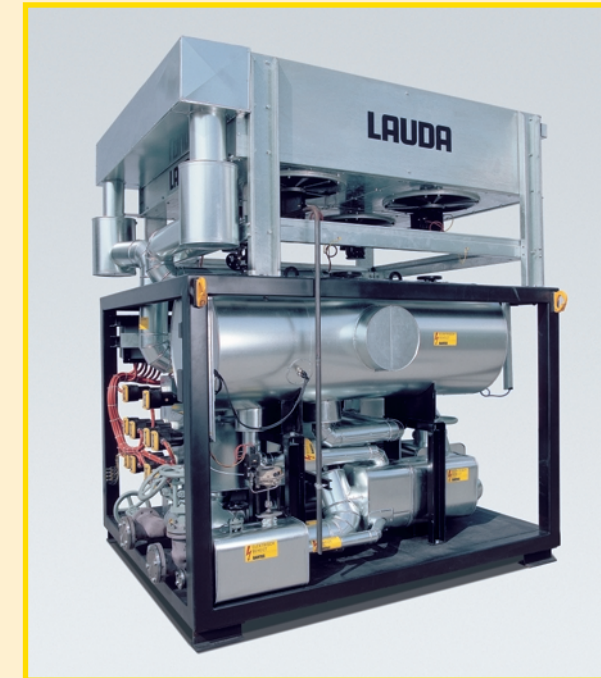
Heat transfer unit with air-cooled heat exchanger for the temperature control of a 20 m 3 reactor in a temperature range from 20 up to 300 °C for installation in hazardous areas. Heating capacity 250 kW Cooling capacity 300 kW at 80 °C Type ITH 600 Ex
