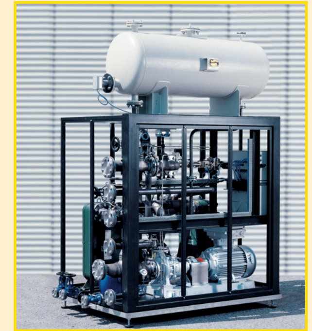
Secondary circuit unit for installation in hazardous area; with two heat exchangers; for the temperature control of a 6300 litre reactor; operating temperature from 40 up to 180 °C Primary energies Steam 200 °C/Cooling water 20 °C Type TR 600 HK Ex
