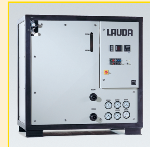
Kryoheater with water-cooled condenser for temperature control within a temperature range from -50 up to 200 °C; equipped with possibility to connect the chilling module LN 2 -Kryopac. Cooling capacity 10 kW/-40 °C Electric heater 48 kW Chilling capacity 10kW/-100 °C Type Kryoheater KH 400 W
