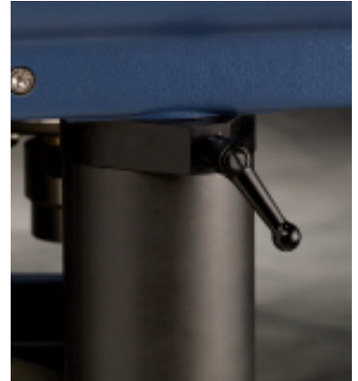
Head position Locator Stop Handle allows specimens to be located at the same position over the platen every time.
