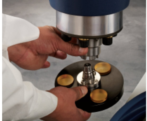
Quick release lift lock chuck provides quick connection and removal of specimen holders.
