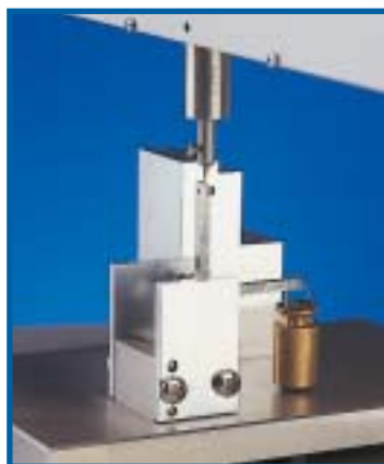
Automatic load cartridge calibration using traceable weights.
