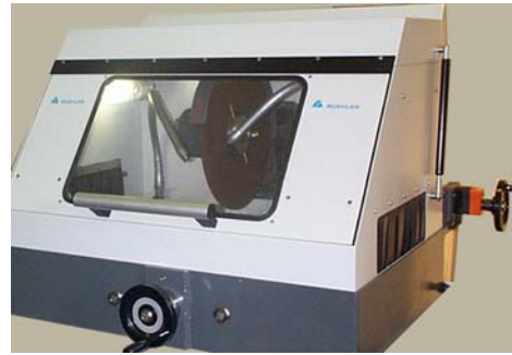
Foreground: Rotating handle for table movement Right, rear: Handle for x-positioning of the cutting arm
