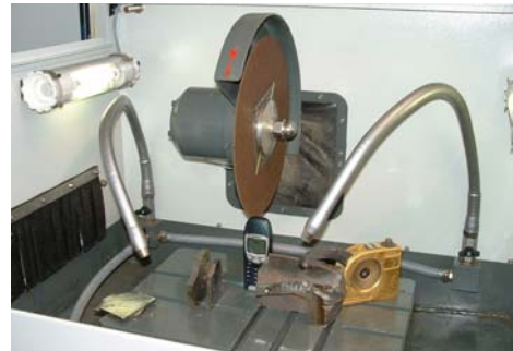
Large Cutting Chamber: Motor and mechanical components of the cutting arm are found outside (behind) the cutting chamber.
