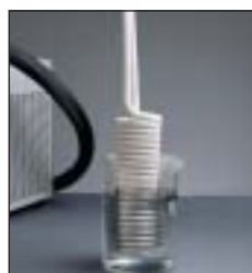
The Probe Coil used in the KR Immersion Series provide to temperature as low as -45^{\circ}\text{C} .
