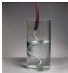
The Flexible Cooling Probe used in the VLT Immersion Series provide to temperature as low as -100^{\circ}\text{C} .
