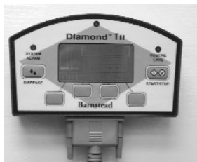
Control Panel Mounted in Remote Location
