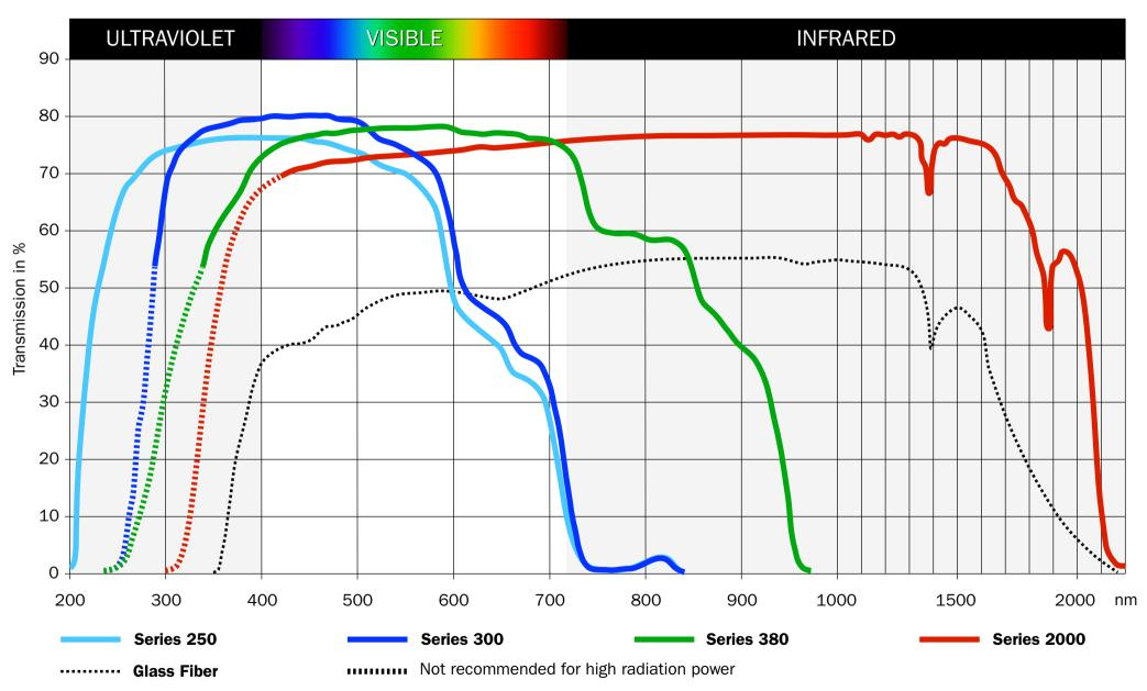
Measured with  $2\alpha=50^{\circ}$  (Series 250  $2\alpha=34^{\circ}$ ), length 2000 mm, active core Ø5 mm
