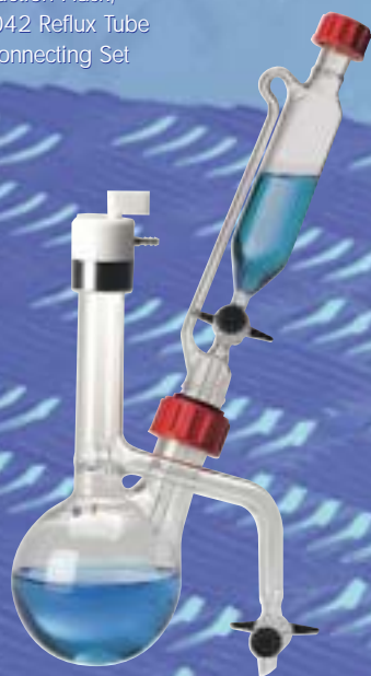
RR99056 - 250ml Azeotropic Reaction Flask with Sidearm with RR99048 - 50ml Liquid Additions Dropping Funnel
