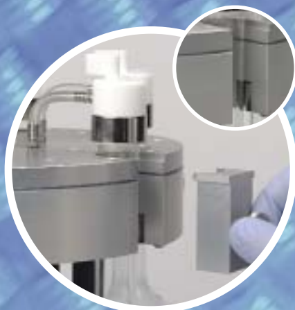
Aluminium inserts allow easy removal of flasks and good heat transfer for efficient refluxing
