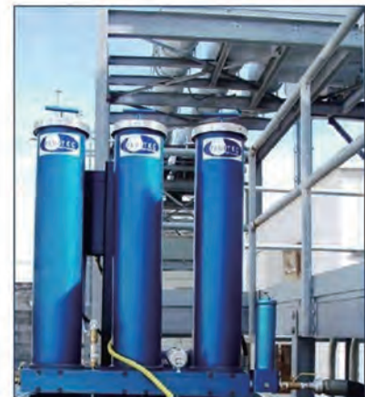
ESP-336 being rotated around a combined cycle plant to maintain 4 turbine oil reservoirs
