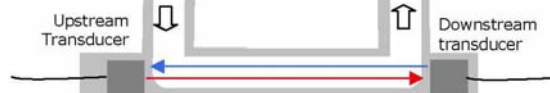
In the micro-flow transducers signal travels squarely with regards to the flow and the travel distance is longer
