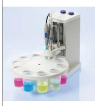
SevenExcellence supports the Rondolino sample changer for methods and series, making automated or unassisted analyses possible. This not only gives you the possibility to focus on other tasks but also allows for special applications such as automated pH calibration.
