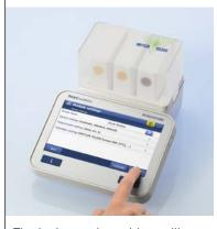
The instrument provides calibration support on many levels, featuring methods with a fixed calibration sequence, automatic evaluation of the calibration results with optional rejection and monitoring of the sensor's age and calibration interval. Automatic calibration with the Rondolino sample changer is also possible!
