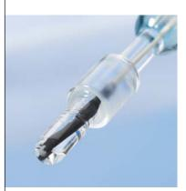
SevenExcellence offers the possibility to check the performance of a pH sensor. The special method type sensor test guides the user through the individual steps, checking various measurement characteristics of a sensor, such as drift and repeatability.
