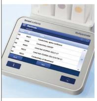
In addition to being more secure, more reproducible due to identical settings and more convenient, methods also enable you to run special applications for conductivity. These include USP/EP measurement of pure water with limits monitoring and Conductivity Ash measurements according to two ICUMSA regulations.
