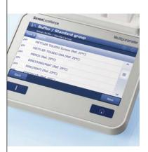
Choose from one of eight pre-defined calibration buffers groups or easily create your own. With the Pick-and-Mix<sup>™</sup> feature you can conveniently combine pH buffers from different groups. After calibration the sensor icon shows you the quality of the calibration at a glance.
