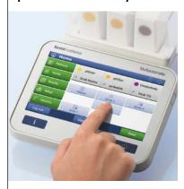
By a single click on a shortcut you can start a method: a sequence of analysis steps with fixed pre-set parameters. Using methods makes sure that your particular analysis is always performed with identical settings.
