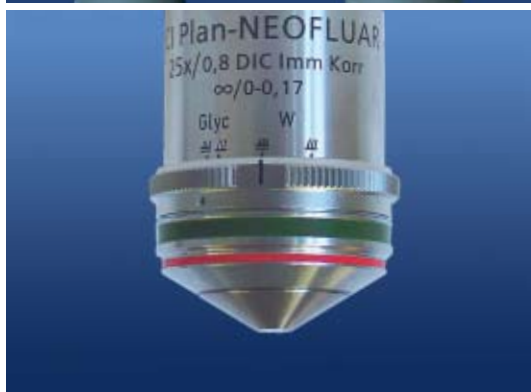
LCI Plan-Neofluars: With temperature compensation for living specimens.
