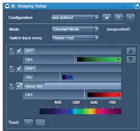
The Imaging Setup Tool displays the detection bands and the selected laser lines for a clear overview of the experiment. Example of a configuration for detecting DAPI (blue), GFP (green) and Alexa 568 (red).
