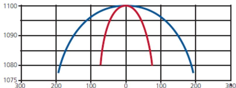
HST 12/200  $\pm 5^{\circ}\text{C}$  over 100mm (mm) HST 12/600  $\pm 5^{\circ}\text{C}$  over 300mm
