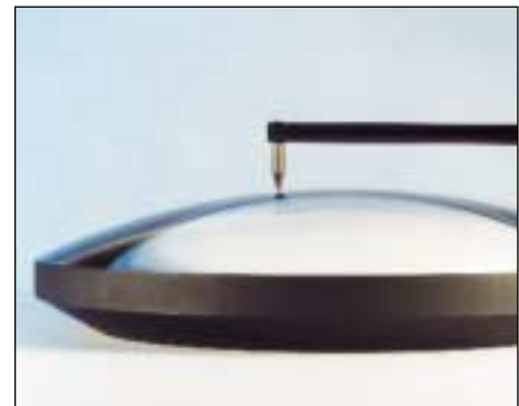
horizontal measuring range is 200mm for single large components or multiple small ones using "step and repeat" program mode
