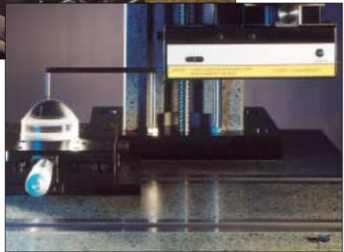
stiffness of the extended length stylus arms makes possible expansion of the range to 25mm or 38mm (shown with 120mm arm for 25mm gauge range)
