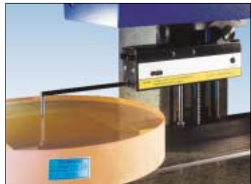
an optical flat is used to calibrate horizontal straightness of the 200mm traverse unit which serves as an absolute reference datum
