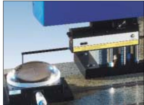
the 80mm spherical calibration standard checks linearity over the entire gauge range and verifies that stylus tip geometry is correct
