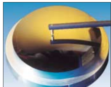
0.8nm vertical and 0.125um horizontal resolution is essential for checking optical quality surface finish on curved components
