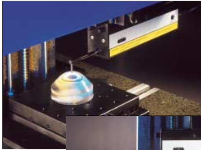
contact of the stylus with the component can be centralized to the rigid, composite granite column for maximum stiffness of the measuring loop
