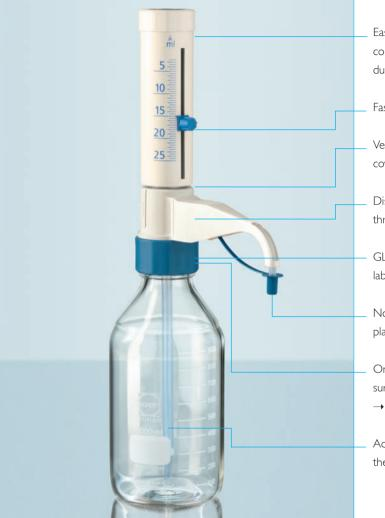
Easy handling thanks to directly pushed piston complete with PFA sealing lip  $\rightarrow$  prevents sticking due to crystal formation
