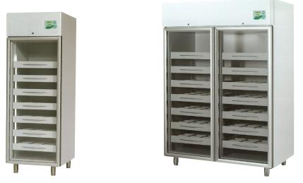
The Emoteca Twin series are similar to the Emoteca range detailed on page R-5, however they feature twin refrigeration systems for added security. This twin system works with two autonomous cooling circuits which alternate during normal operation cycles to maintain the set temperature.
