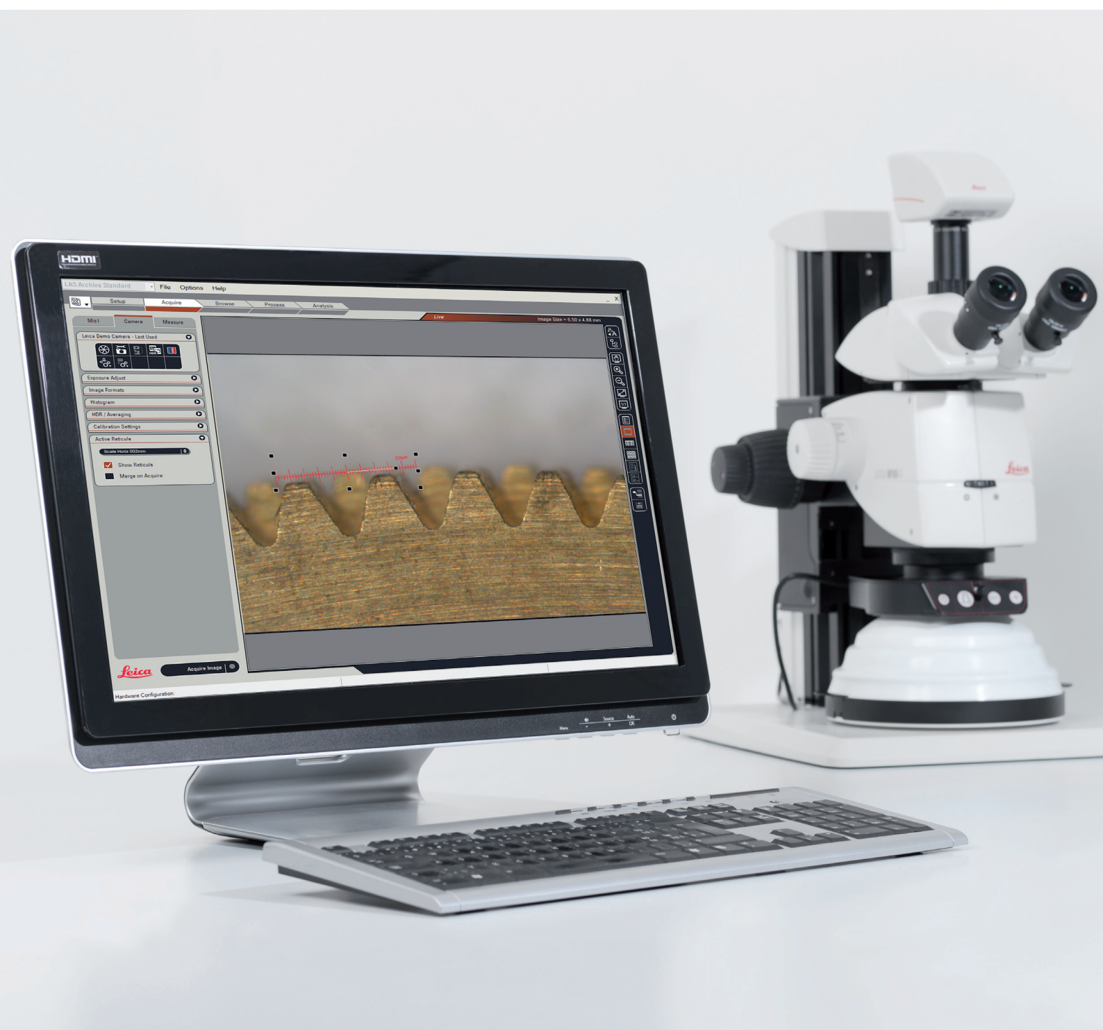
Reticule to estimate component symmetry and diameter.
