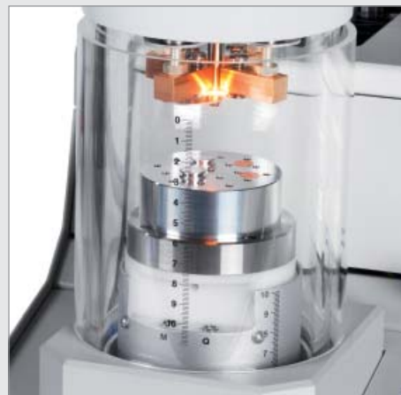
The CEA050 Carbon Evaporation Accessory module is easy to mount either with a single or multiple carbon thread evaporation flange. The carbon thread is covered during the degassing process by a shutter which protects the specimen from damaging heat and impure carbon coating. A standard height adjustable table ensures specimens of varying sizes are set at the optimum distance from the carbon evaporation source. Excellent for preparing films for X-ray microanalysis or carbon reinforcement films for TEM specimen support grids.
