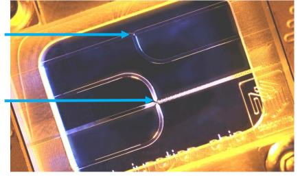
Many common emulsions are formed as either "oil droplet in water" or "water droplet in oil". In each case, it is important that the flow channels have the correct hydrophobic or hydrophilic properties to promote droplet formation. This is readily achieved either by selection of an appropriate primary substrate for example hydrophilic glass or hydrophobic polymer. Alternatively surface properties and contact angle can be modified by a coating process.
