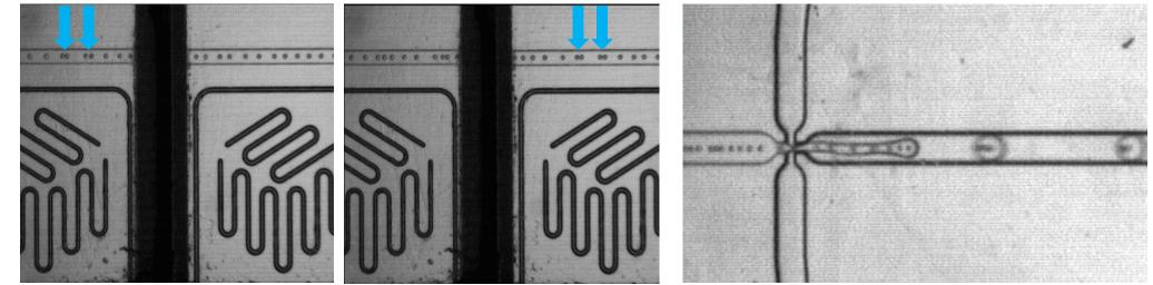
Fluid flow details: Aqueous inner droplet flow: DI Water 0.4 to 1.0 µL/min Oil droplet phase: Medium Chained Triglyeride with 1.25% PGPR surfactant @ 25 to 50 µL/min Water sheath phase: DI water with 0.2% whey protein isolate @ 250 to 350 µL/min
