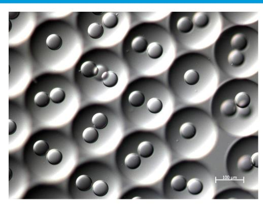
Adjustment of the three flow rates was performed to observe the range of droplet sizes that could be created. Although further work is continuing in this area, and not all combinations of inner and outer droplet diameter can be achieved with a single chip pair, it is possible to achieve inner droplet diameters in the range 25 to 50  $\mu$ m and outer droplet diameters of 150 to 200  $\mu$ m.
