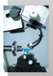
The Adjustable Antistatic electrode is a helpful accessory for sectioning at room temperature.
