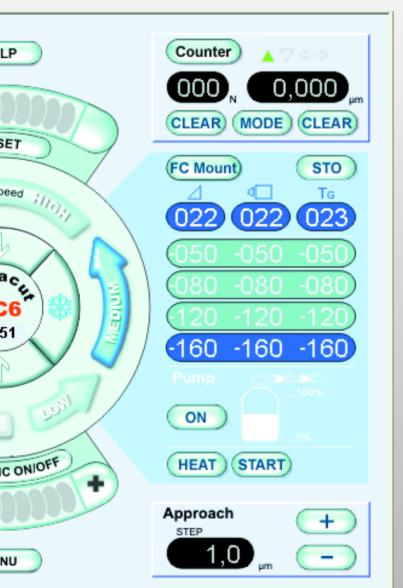
The FC Mount function and the threaded hose connector allow you to mount and dismount the FC6 chamber within seconds. Connection and Disconnection of Hot Plugs can be carried out while the instrument is connected to the mains.
