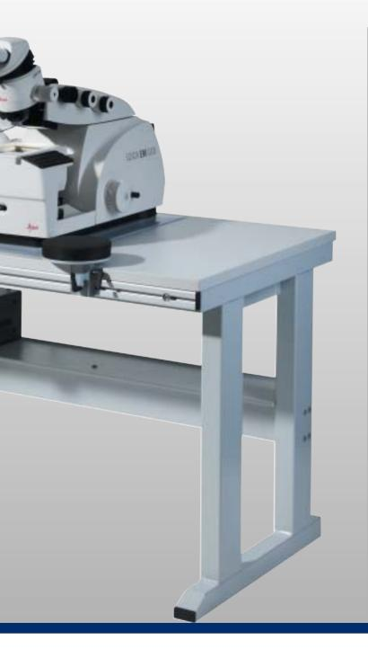
The EM FC6 cryo ultramicrotome is designed for state-of-the art biological, clinical and industrial applications.
