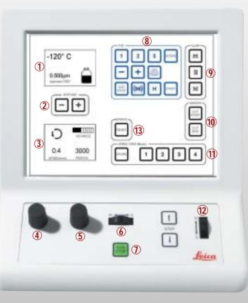
**E-W coarse wheel** allowing 25 mm travel of the knife stage left and right.
