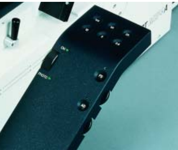
Armrest with integrated keyboard of the Mef4
