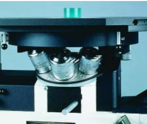
Motorized sextuple turret carrying the high quality lenses
