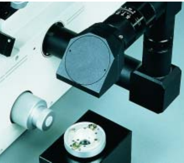
MacroDual Zoom attached on the left hand side of the stand
