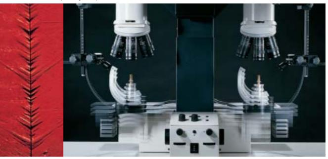
Motorized control of x/y/z for single and synchronous movement.
