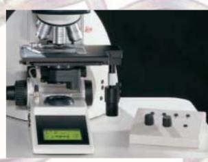
Stand-alone control panel of the Leica FS4000.
