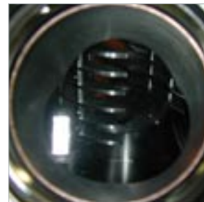
Side view on the wafer storage module for up to six 4" wafers.
