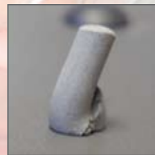
The same test with 20 g load leads to an irreversible deformation of the sample
