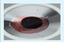
Many samples have air trapped inside them or are carbonated. These samples read well most of the time as long as air bubbles are not trapped between the prism surface and the sample. When this happens the operator gets an erroneous result often referred to as a flyer. These results are called flyers because the measured value is quite different from the expected measurement value.
