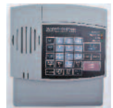
Sensaphone Telephone Dialing System
