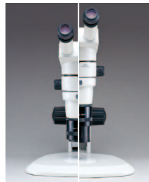
Ergonomic objective can be extended or retracted to adjust eye level.
