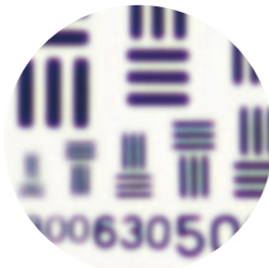
Resolving power chart SMZ1500 with P-HR Plan Apo 1.6x objective
