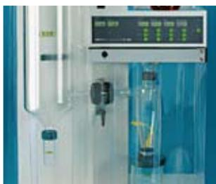
If no fume hood is available and work is being carried out with inflammable or toxic products, the safety curtain is a highly reliable alternative. It is easy to unfold and the lamella permit inspection and access to the glass elements whilst the spray drying process is underway (incl. in B-290 Advanced).
