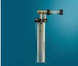
Outlet filter with a polyester-deep bed filter and display of the pressure drop. Provides optimal protection for the aspirator and whilst permitting cleaning of the aspirator. The additional filter, made of a porous PTFE-membrane, also facilitates the recovery of the product by means of compressed air counter-pulses. A filter bag for each is included.
