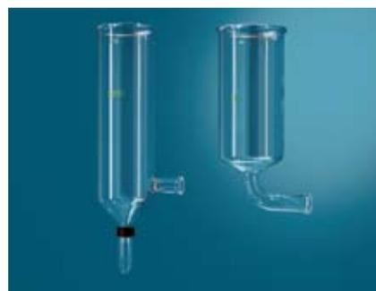
Two different versions of the glass cylinders make it possible to optimize the yield depending on the process. The lateral outlet cylinder is particularly suitable for aqueous products which are difficult to dry, whilst the second type of cylinder with a vertical outlet geometry is especially useful for work involving organic solvents.
