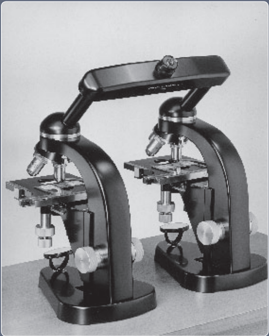
Monocular comparison microscope by Ernst Leitz, Wetzlar, year of construction 1955
