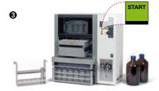
The protective shield is closed, the cells sealed automatically and 6 samples are extracted at the push of a button.
