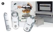
The flexible sealing system in the Multi-vapor makes it possible to individually seal different collection bottles (60, 150, 220 and 240 ml). Cross-contamination is therefore excluded.
