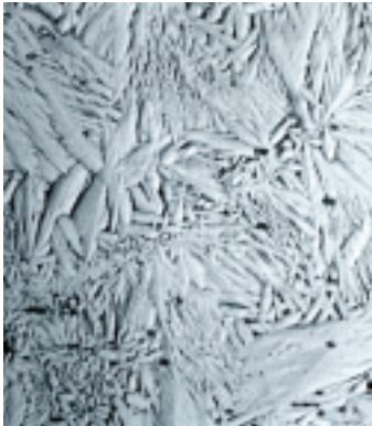
Nitinol martensitic structure after going through the shape memory effect at 1000x.
