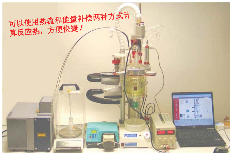
BRUKER IR 电子天平 蠕动泵 Atlas Potassium 补偿电源 Atlas Software
