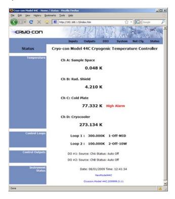
The TCP/IP data port server brings fast Ethernet connectivity to all common data acquisition software programs including LabView™. TCP/IP implements an ASCII text based command language similar to those commonly used with GPIB or RS-232 interfaces. This is the primary way that user software interfaces to the instrument.
