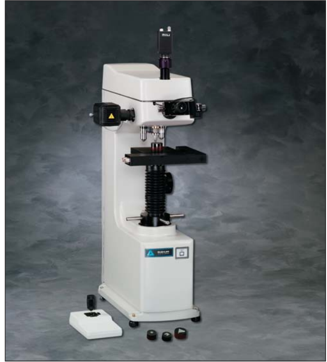
MacroVickers model 1900-5114 with motorized stage and joystick control for semi-automated operation.
