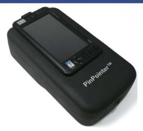
The *PinPointer*<sup>TM</sup> packs a full-featured Raman spectroscopy system in a remarkably affordable true handheld format. The lightweight unit is controlled by a pocket-size Windows® computer and features easy-to-use *RSIQ*<sup>TM</sup> software for fast point-and-click operation. An optional software module add-on *RSIQ-QUAL*<sup>TM</sup> provides one-touch identification of unknown substances by immediate comparison of a measured spectrum to the on-board Raman spectral library.
