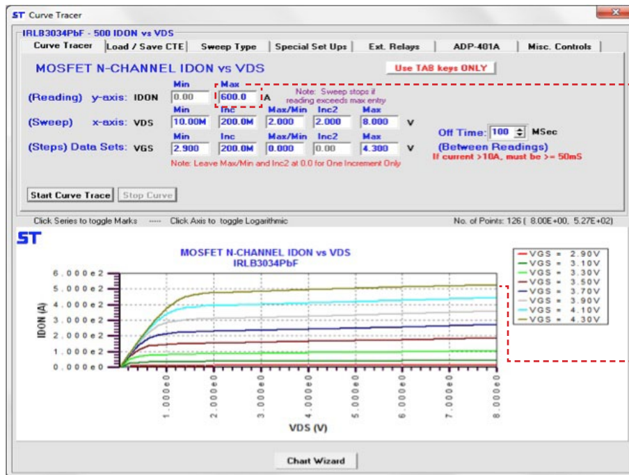
HI Current MOSFET, ID vs VDS (Figure 4)
