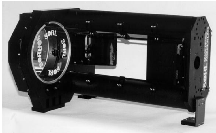
4 Mirror Afocal Telescope shown with the Protective Covers Over the Primary and Tertiary Mirrors
