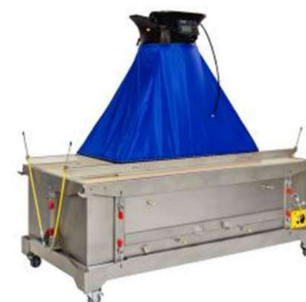
Integral flow hood measurement
