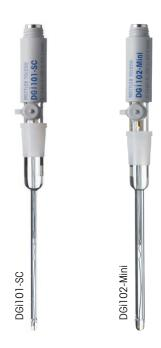
The DGi101-SC and DGi102-Mini are two powerful micro pH sensors with 3 mm or 6 mm shafts especially made for small sample volumes of 5 to 20 mL and for use on the InMotion Autosamplers with 80 mL or 25 mL beakers. With the moveable sleeve holder, the height can be adjusted. Samples containing sulfides can be titrated with no problem. The ARGENTHAL™ reference system with silver ion trap means there is no possibility of diaphragm clogging.
