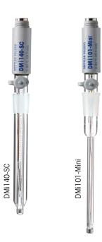
The DMi140-SC and DMi101-Mini are two platinum ring sensors for all types of redox titrations encountered in the electroplating or electronics industries, such as direct titration with cerium(IV)sulfate or back titrations with potassium iodide or ferrous(II) ammonium sulfate. The DMi140-SC is the generalist while the DMi101-Mini is a rugged semi-microsensor for small sample volumes of 10 to 20 mL or for use on the InMotion Autosamplers with 80 mL and 25 mL beakers.
