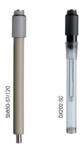
This is a specific combination for acid-base titration in media containing hydrofluoric acid. The antimony pin of the Sb850 half cell is passivated by fluoride ions and is therefore resistant. Similarly, the plastic shaft of the DX202-SC reference is unaffected by hydrofluoric acid. Oxides that are only soluble in highly corrosive media can be titrated without any trouble.
