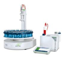
The METTLER TOLEDO InMotion Autosamplers platform used in conjunction with the Excellence titrators forms exceptionally versatile and high-performance titration systems. It is made possible by the modular design, the intuitive controls and the Plug and Play hardware. This means you can configure your day-to-day titrations with ease, start them at the press of a button and let them run automatically without intervention.
