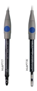
These two conductivity sensors, which can be connected directly to the conductivity card of an Excellence titrator, are suitable for conductometric acid-base or precipitation titrations. They can be used in low-ion aqueous or non-aqueous media. They enable rapid titration and feature zeromaintenance and outstanding durability. For direct measurement of conductivity, the appropriate InLab®710/731 or InLab®720/741 can be used according to sample type.
