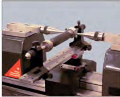
测量螺纹塞规 HPA-1/TEL6/3P/0.17-3.2/S6.5 / LABC-15
