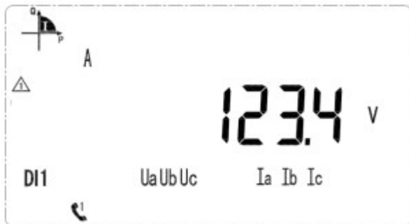
Voltage on A phase is 123.4V
