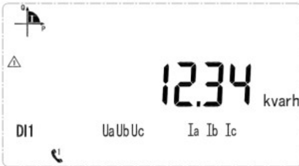
Current forward reactive energy 12.34kWh
