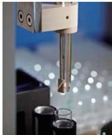
Five miniature probes entering sample vial
