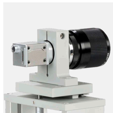
LMO 0103 Telecentric lens of the LSA 100 Research
